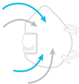
Inhalation with a 3M™ Cool Flow™ Valve
