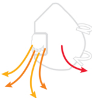
Exhalation with a 3M™ Cool Flow™ Valve
